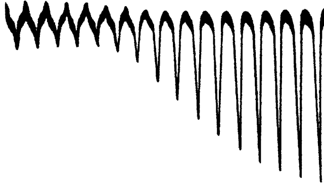
Figure 4.14 Oscillogram of core saturation process for great value \Delta I_y .
